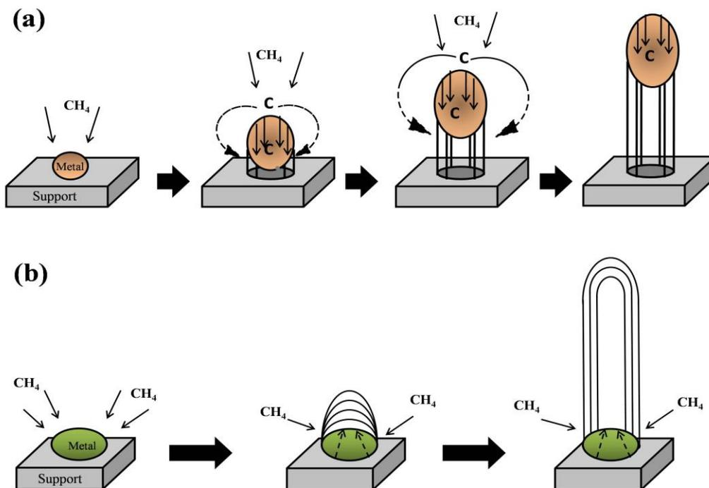
Figure 2: Growth mechanism of MWCNTs
