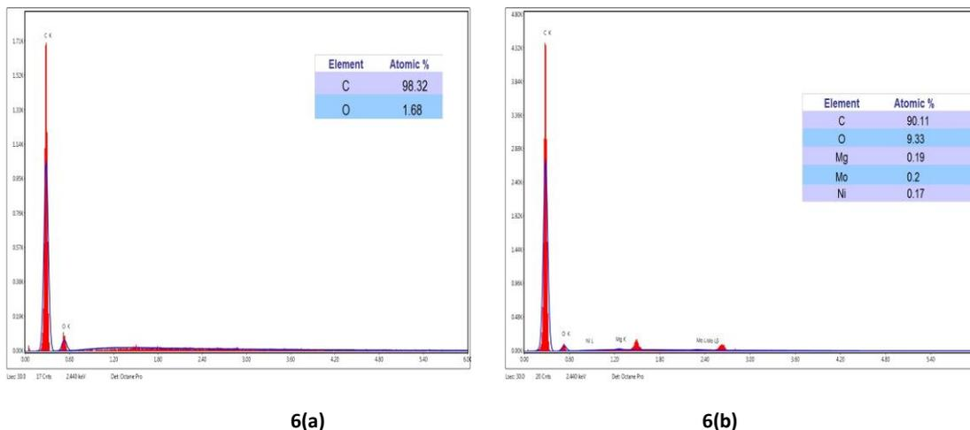
figure 6: EDX of the prepared MWCNTs over (a) Fe-Mo catalyst, and (b) Ni-Mo catalyst.
